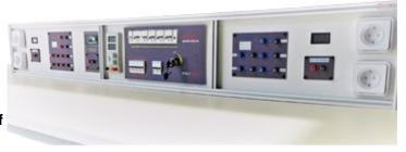
The bench consists of a **lab bench PT 3000 B** and the **single side Power Supply Unit PT 3000 BE**. The standard configuration of the PT 3000 BE is provided below.
